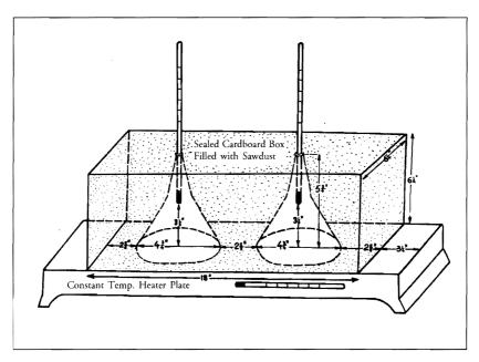
Figure 1. The apparatus used in this study involved 2 funnels, a metallic one and a plastic one, sitting in a cardboard box filled with sawdust. Thermometers were passed through the neck of each funnel, positioned as indicated in the figure, and attached to the stem with adhesive tape. The cardboard box was positioned on a heating plate whose temperature could be raised from room temperature to  $50^{\circ}C$  and lowered back to room temperature.
