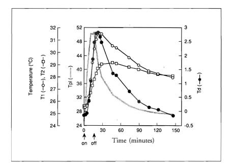
Figure 2. The effect of raising the temperature of the heating plate (Tpl) to 50°C, and then immediately lowering it back to room temperature, on the temperature of the air in the metallic funnel (T1), the air in the plastic funnel (T2) and the temperature difference between them (Td).
