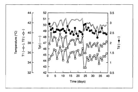
Figure 3. The variation of the temperature of the air in the metallic funnel (T1), the air in the plastic funnel (T2) and the temperature difference between them (Td) when the box containing the funnels was maintained continuously on a heating plate set at 50°C for 39 days.
