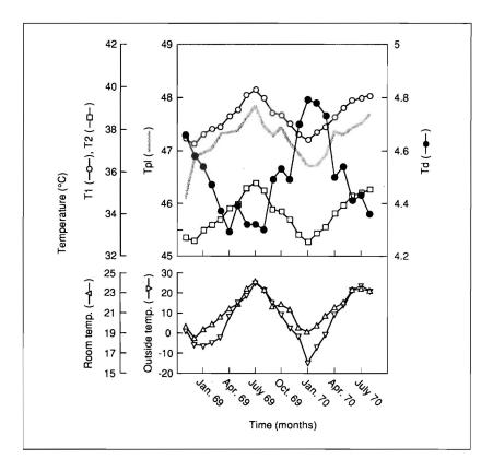
Figure 4. The variation of the temperature of the air in the metallic funnel (T1), the air in the plastic funnel (T2) and the temperature difference between them (Td) when the box containing the 2 funnels sat for 22 months continuously on a heating plate set to heat to  $47^{\circ}C$  (Tpl). Room temperature and outside temperature are also included in the figure.
